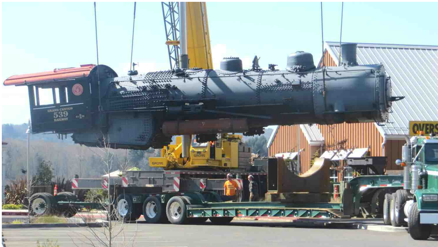
The Boiler for SP&S 539 / NP 1762 is lifted from the Trailer - Photo by Arlen Sheldrake
