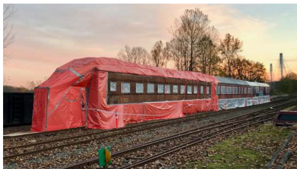
Cars Wrapped for Decontamination
