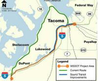
Passenger trains, including Amtrak Cascades, must slow down due to curves and single-track tunnels on the BNSF Railway main line tracks (green line) near Point Defiance and along southern Puget Sound. This project will reroute passenger trains to a bypass rail line along I-5 (orange line).
