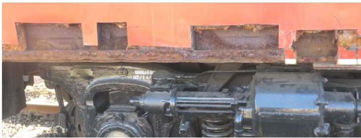
Inspection cuts on the No. 6800 to determine extent of required repairs
