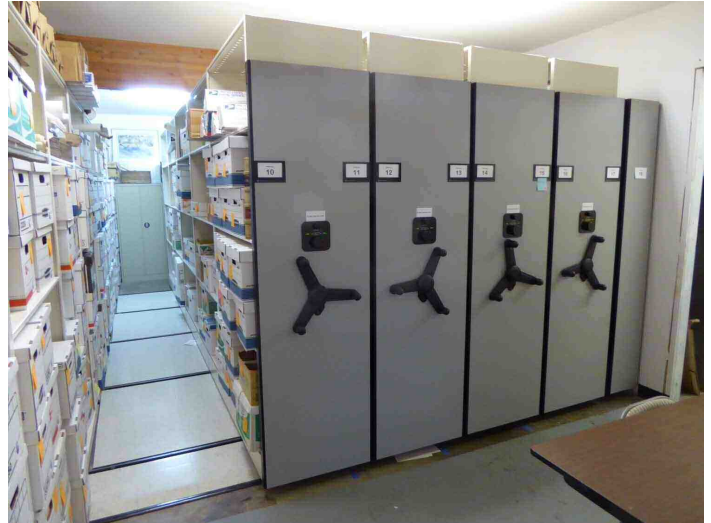
The mobile shelving carriages in the Archive's mid-bay have now been extended to the full 88-inch allowed height.
