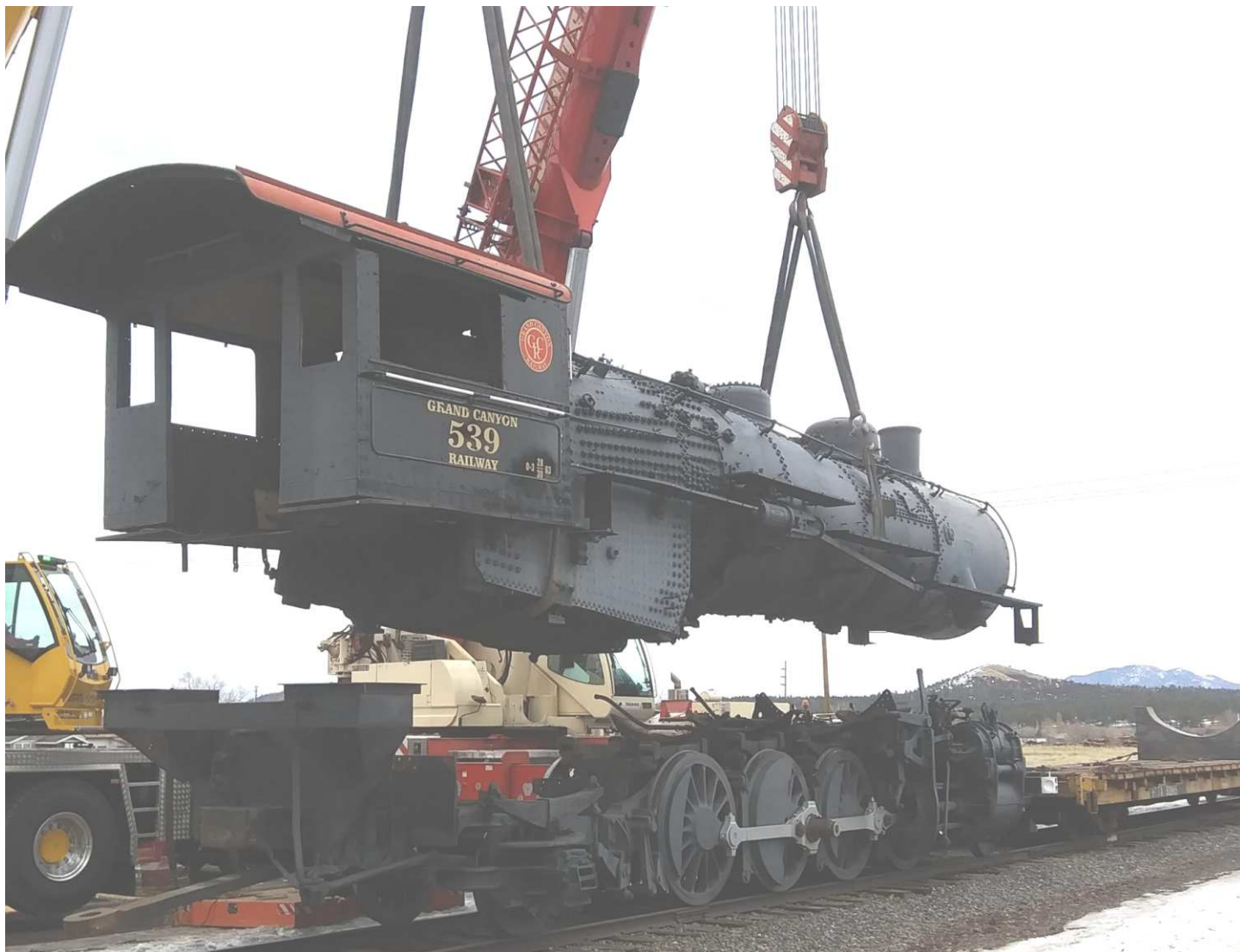
The NP No. 1762 (SP&S No. 539) Loaded onto Flatcars by Wasatch Railroad Contractors - Port of Kalama Photo
