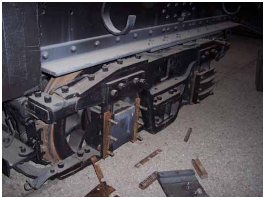
Over the total production run, the Willamette truck changed several times. The spoked wheels are clearly shown in this fireman's-side view. Photo: Steve Hauff
