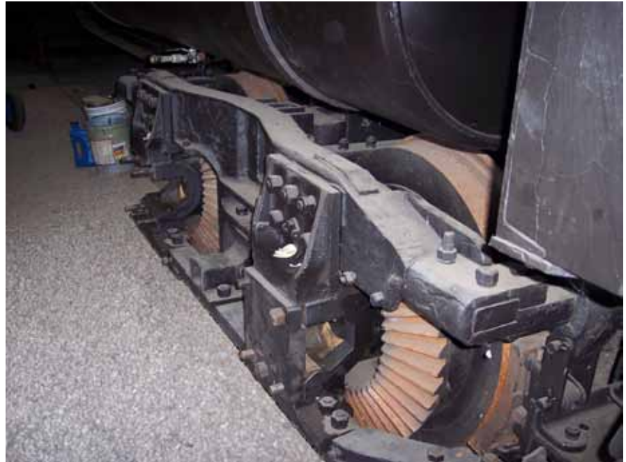
Shown here without the line-shaft, the Willamette truck was of the cast style. The cast trucks tended to be more rigid, and required less maintenance, than the archbar design used on many Shays. Photo: Steve Hauff
