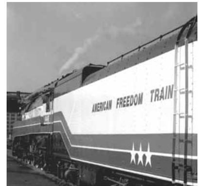
Inviolate were the 13 display cars that were mechanically and electrically connected. Each display car had a moving sidewalk down one side and the only way to pass through the train was from the entrance car. Not having 969 feet of continuous length meant the train could not stop in the town. Also, the showcase cars could only be so many feet from the generator car since they had to be electrically connected to the train's main generator.
