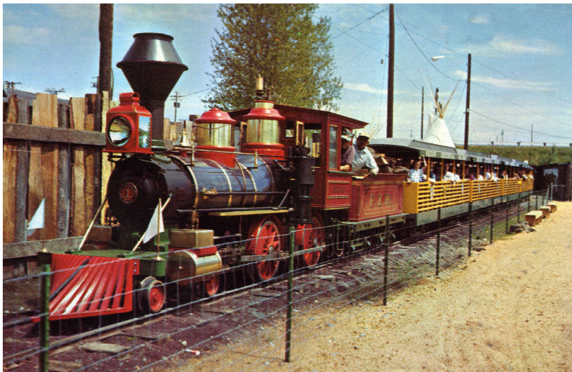
Below: The Oregon was designed to operate on very sharp curves as illustrated by the front wheel being well outside the pilot (cowcatcher).
