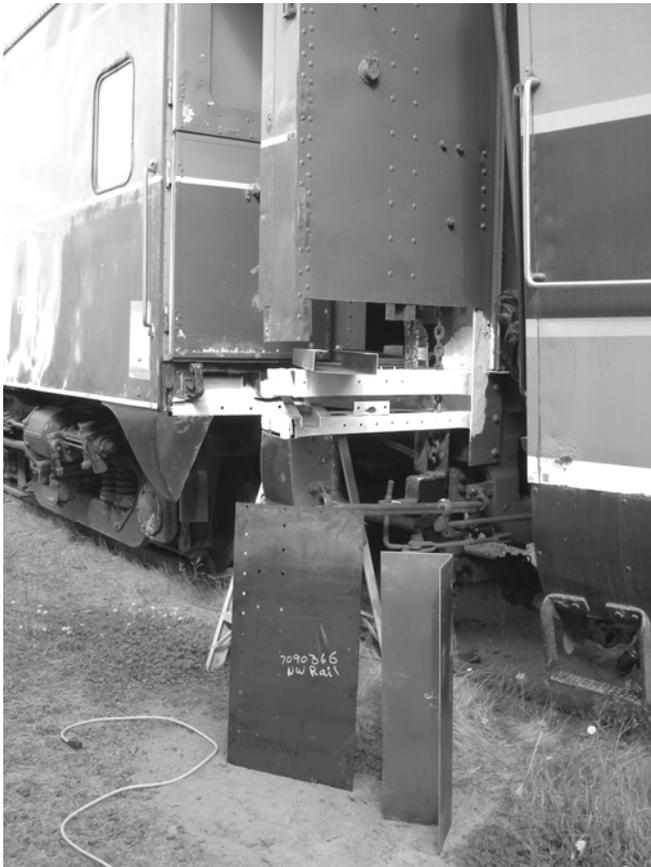
On September 23<sup>rd</sup> work progresses on the Chapter's Red River 6800 coach as Keith Fleschner and Pete Rodabaugh work to replace the rusted metal in the vestibule. The vestibule stairs have been removed. The new metal is displayed and the remaining metal has been sandblasted and painted.
