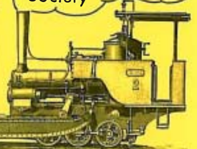
This remarkable double locomotive was the product of Charles Brown and featured a lever drive. It was built in 1878 at Brown's Winterthur factory for the narrow-gauge Villa Real and Villa Regoa tramway in Portugal. (Recent Locomotives, Fig. 175)
