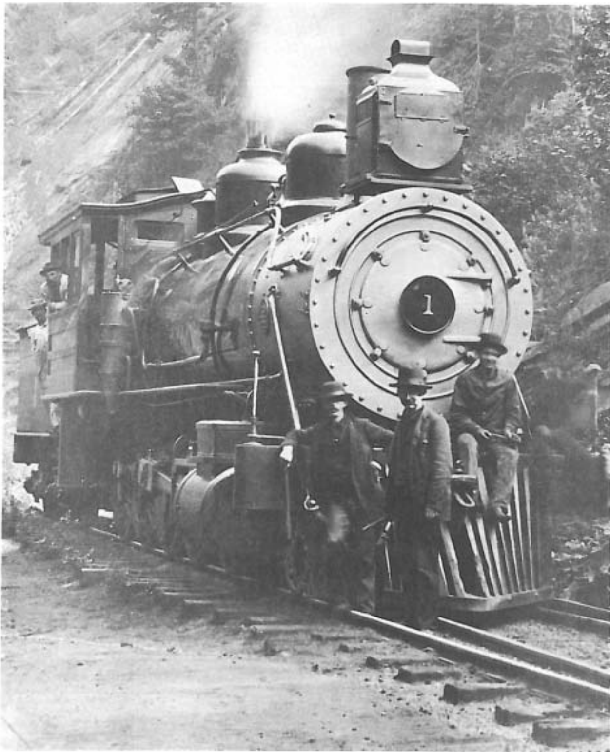
NP Engine #1 (2-10-0) near Wilkeson, Washington about 1900. Engines #1 & 2 were built in 1866 for use on the switchback. These were believed to be the largest of their type when built.
